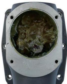
**Figure 3 new grease example
