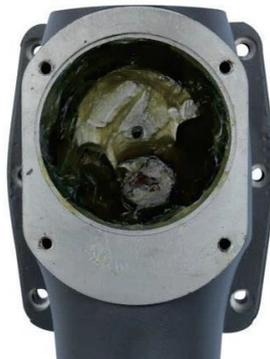
**Figure 2: Grease ring example**
