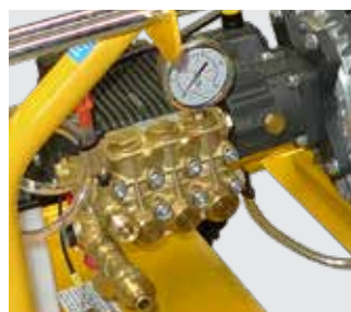
TRIPLEX PUMP WITH 2:1 REDUCTION GEARBOX
