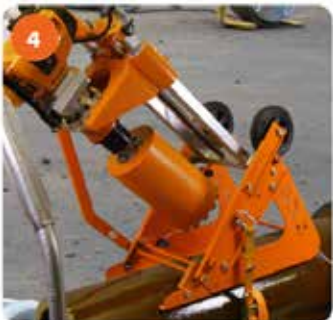
45° Drill in cast iron pipe. Fixing by strap, clamping ratchet and angle support (accessory).
