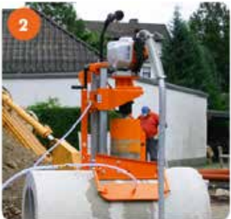
45° Drill in cast iron pipe. Fixing by strap, clamping ratchet and angle support (accessory).
